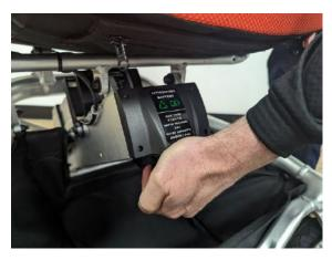
To remove the primary battery, pull the release lever up and slide the battery towards you.
