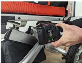
To remove the secondary battery, pull the release lever up and slide the battery towards the front of the chair and then rotate it outwards and pull towards you.
