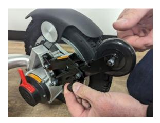
Fold the anti-top wheels in by pulling out the adjustment knob and pushing them up and towards the chair.
