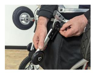
To open the climber wheels, pull the release knob out and lift each climber wheel up until it locks into position.
