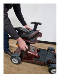
4. Place the seat back into the seat base, push the seat rotation handle down and ensure it is securely in place before use.
