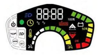
Your Connex scooter is equipped with an LED display. The green light indicates that the device is turned on. The headlight symbol indicates the headlight is turned on. The battery indicator runs round the right-hand side of the display. Your speed will be indicated round the speed adjustment knob.
