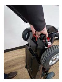
5. To remove the rear section, use the red lever and pull the rear black bar upwards until the section is removed.
