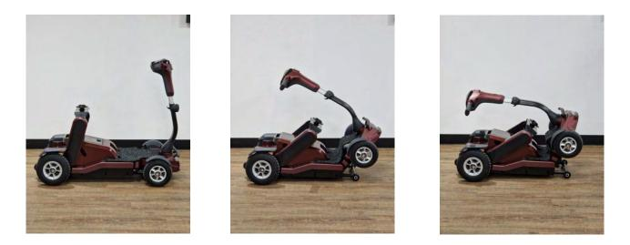
3. The scooter will then begin its electronic folding function. This process should take roughly 15 seconds.
