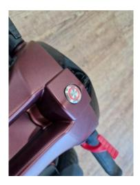
2. Press the fold/unfold button on the tiller of the scooter to begin the electronic fold function. Please note you may need to press this twice to start this function if the scooter has been off for more than 2 minutes.
