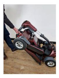
4. If required, use the black handle on the rear of the scooter to lift the folded scooter into its upright position.
