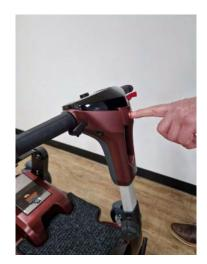
2. Press the fold/unfold button on the tiller of the scooter to begin the electronic fold function. Please note you may need to press this twice to start this function if the scooter has been off for more than 2 minutes.
