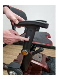
To adjust the height of the armrests, press the silver button on the side of the armrest and adjust height. Release the button and ensure the armrest is locked in place.
