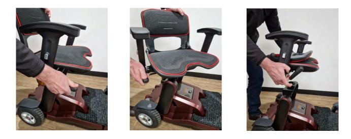
1. Push the seatback down, then push down the seat rotation lever and lift the seat upwards to remove it.
