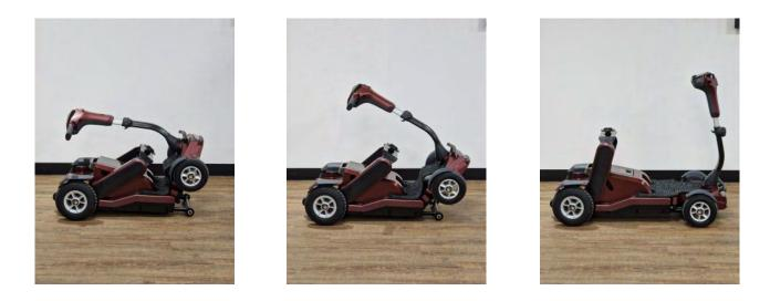
3. The scooter will then begin its electronic unfolding function. This process should take roughly 15 seconds.
