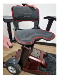
The collapse the armrest, press the small silver button just above the orange reflector. The armrest can then be collapsed. Please note, the armrest only has two locked positions – upright and fully collapsed.
