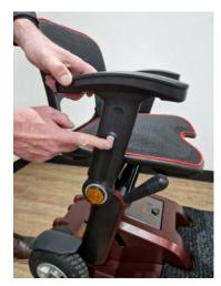
To collapse the armrest, press the small silver button just above the orange reflector. The armrest can then be collapsed. Please note, the armrest only has two locked positions – upright and fully collapsed.
