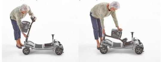
Lift up the tiller by first loosening the tiller adjustment knob and then slowly lifting the tiller up away from the floorpan. Once the tiller is upright then tighten the tiller adjustment knob to keep it in place.
