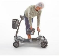
Using the handle on the battery lift up to remove the battery pack. Be aware the battery is secured in place with Velcro so if you are struggling to remove it push down on the seat post to help make it easier.
