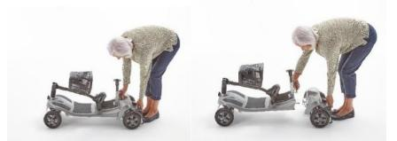
Lift up the rear section removal handle with one hand and pull down the rear section with the handle to separate the front and rear sections. Lift up and away the front section.
