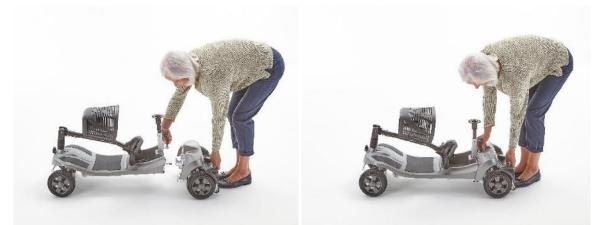
Use one hand to pull down the rear section with the handle and lift the front section using either the seat post or rear section removal handle. Drop the front section into the rear section and push down until you hear a click. Always check that the sections are connected correctly before moving on to the next stage.
