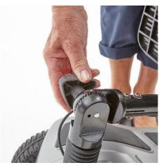
When the tiller is in the desired position turn the tiller adjustment knob clockwise until it is as tight as possible.
