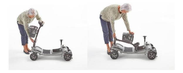
Fold down the tiller by first loosening the tiller adjustment knob and then slowly pushing the tiller down towards the floorpan. Once the tiller is resting on the floor pan the tighten the tiller adjustment knob to keep it in place.
