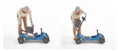
Lift up the tiller by first loosening the tiller adjustment knob and then slowly lifting the tiller up away from the floorpan. Once the tiller is upright then tighten the tiller adjustment knob to keep it in place.
