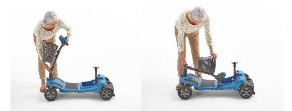
Fold down the tiller by first loosening the tiller adjustment knob and then slowly pushing the tiller down towards the floorpan. Once the tiller is resting on the floor pan the tighten the tiller adjustment knob to keep it in place.
