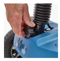
Lock the tiller in place using the tiller lock by pushing the lock in and rotating it 90 degrees clockwise.
