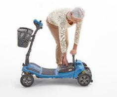
Insert the battery pack into the floorpan. Push down to ensure it is secured.
