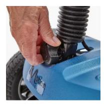
Unlock the tiller by pushing the lock in and rotating it 90 degrees anti-clockwise.
