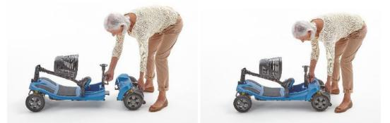
Use one hand to pull down the rear section with the handle and lift the front section using either the seat post or rear section removal knob. Drop the front section into the rear section and push down until you hear a click. Always check that the sections are connected correctly before moving on to the next stage.
