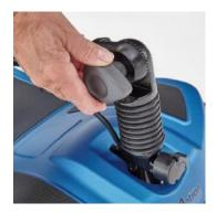
When the tiller is in the desired position turn the tiller adjustment knob clockwise until it is as tight as possible.
