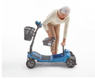
Using the handle on the battery lift up to remove the battery pack. Be aware the battery is secured in place with Velcro so if you are struggling to remove it push down on the seat post to help make it easier.
