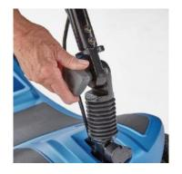
To adjust the tiller, hold the tiller in one hand and turn the tiller adjustment knob anti clockwise with the other until the teeth disengage and the tiller can move up and down freely.
