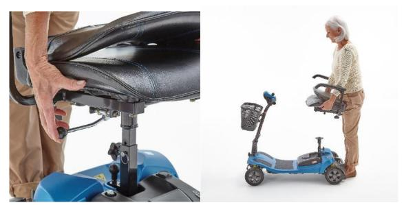
Lift up the seat rotation lever and lift the seat upwards to remove it.
