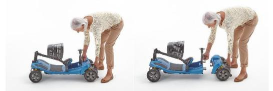
Lift up the rear section removal knob with one hand and pull down the rear section with the handle to separate the front and rear sections. Lift up and away the front section.
