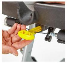
Pull the Yellow handle on the rear of the seat to unlock the seat.
