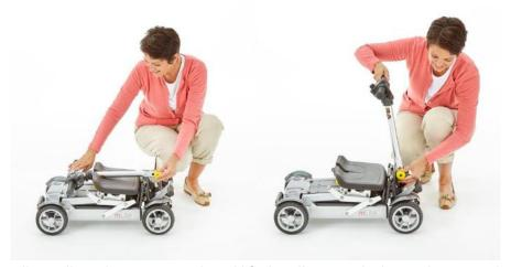
Pull the Yellow Tiller Adjustment Knob and lift the tiller up to lock into the upward position.
