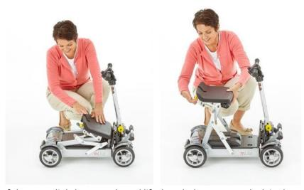
Tip the rear of the seat slightly upwards and lift the whole seat up to lock in the open position.
