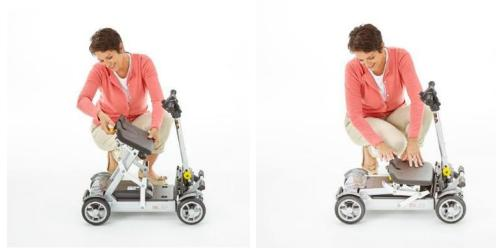
Tip the front of the seat slightly forwards and push the whole seat downwards to lock in the closed position on the floorpan.
