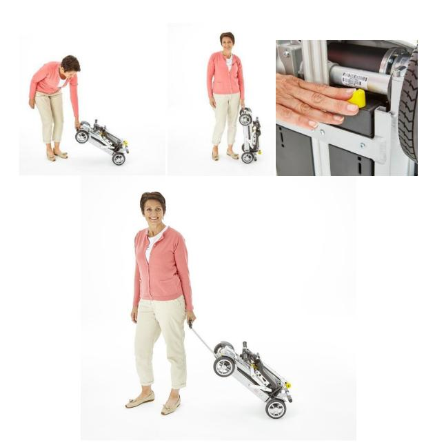
The Scooter can then be lifted and the handle can then be extended to the desired height by pressing the Yellow handle release button to the right and sliding the handle up until it locks into the correct position.
