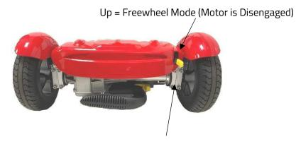
Down = Driving Mode (Motor is Engaged)
