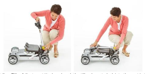
Pull the Yellow Tiller Adjustment Knob and push the tiller down to lock into the seat in the closed position.
