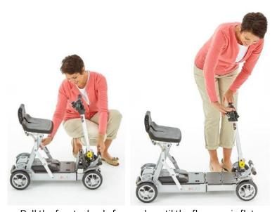
Pull the front wheels forwards until the floorpan is flat.
