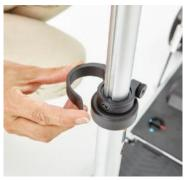
To adjust the tiller height, hold the tiller in one hand and release the Tiller Adjustment Clip until the tiller can move up and down freely.
