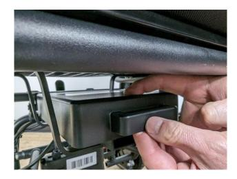
To remove the battery, press the release button and slide the battery towards you.
