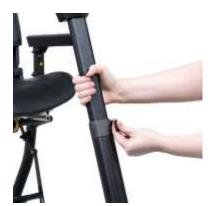
To adjust the tiller, hold the tiller in one hand and pull the tiller adjustment clip and the tiller can then move up and down freely.
