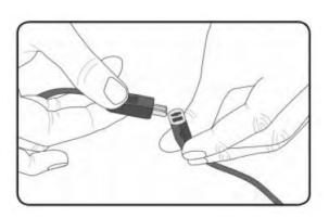
4. At the rear of the chair, connect the base and backrest heat, massage and control functions together by connecting the internal wires (these wires will be loosely protruding from the bottom of the backrest and will be at the rear of the base).
