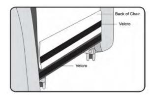
6. Seal fabric from the corner of the seat to the base of the backrest using the Velcro strips.
